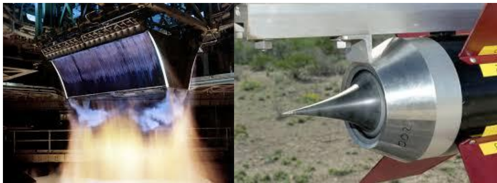
Fig. 8: Examples of linear and toroidal aerospike nozzles [13]
