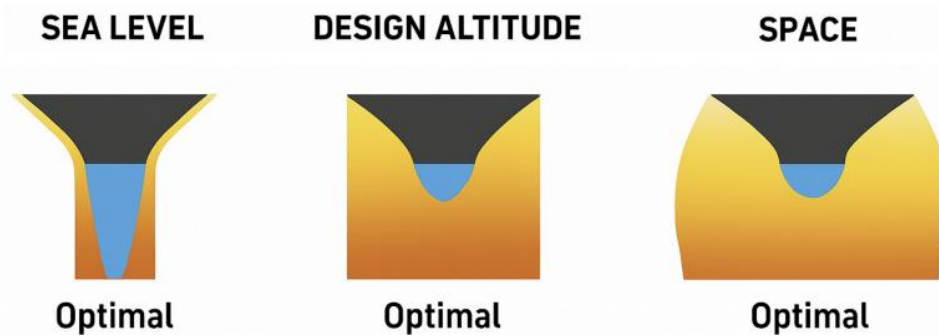
Fig. 9: Expansion of exhaust flow at various altitudes [14]
